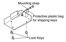
The eject operation cannot be performed if the keys are mounted when the power is turned on. Turn the power off, then remove the keys.
